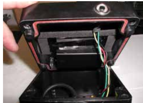
Figure 5. Proper position of lid and wiring
