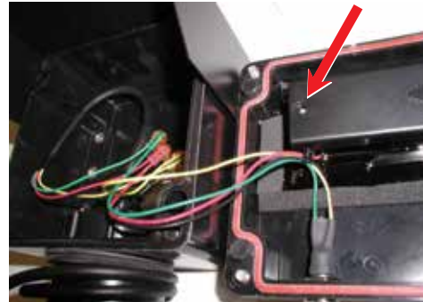
Figure 4. Battery cover and screw
